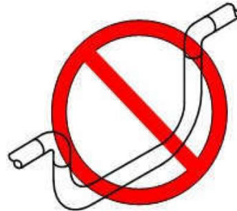
FIGURE 4. - Insufficient Condensate Trap
