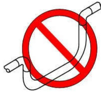
FIGURE 3. - Insufficient Condensate Trap
