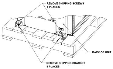
FIGURE 4 - Standard Packaging with Brackets - Back View
