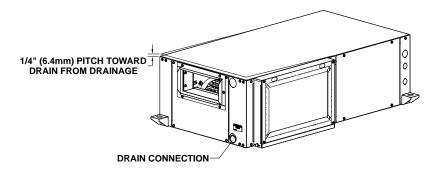
FIGURE 12 - Horizontal Unit Pitch
