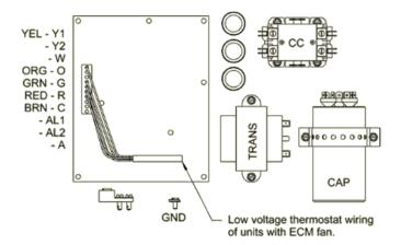
FIGURE 21 – Control Voltage Layout
