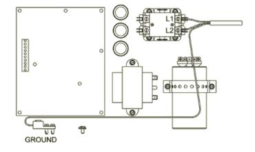
FIGURE 22 - Single Phase Line Voltage Field Wiring
