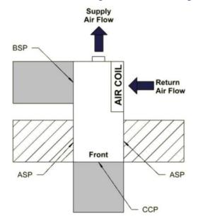
FIGURE 9 – Right Return Straight Discharge
