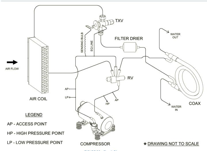
FIGURE 30 - Circuit Diagram
