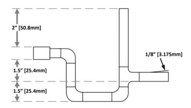
FIGURE 15 – Condensate Drain Layout
