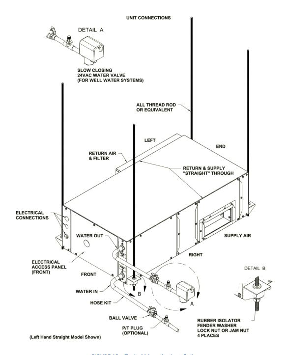
FIGURE 13 – Typical Mounting Installation
