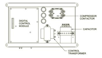
FIGURE 20 - Control Box Layout
