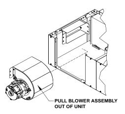
FIGURE 23 - Blower Removal Detail
